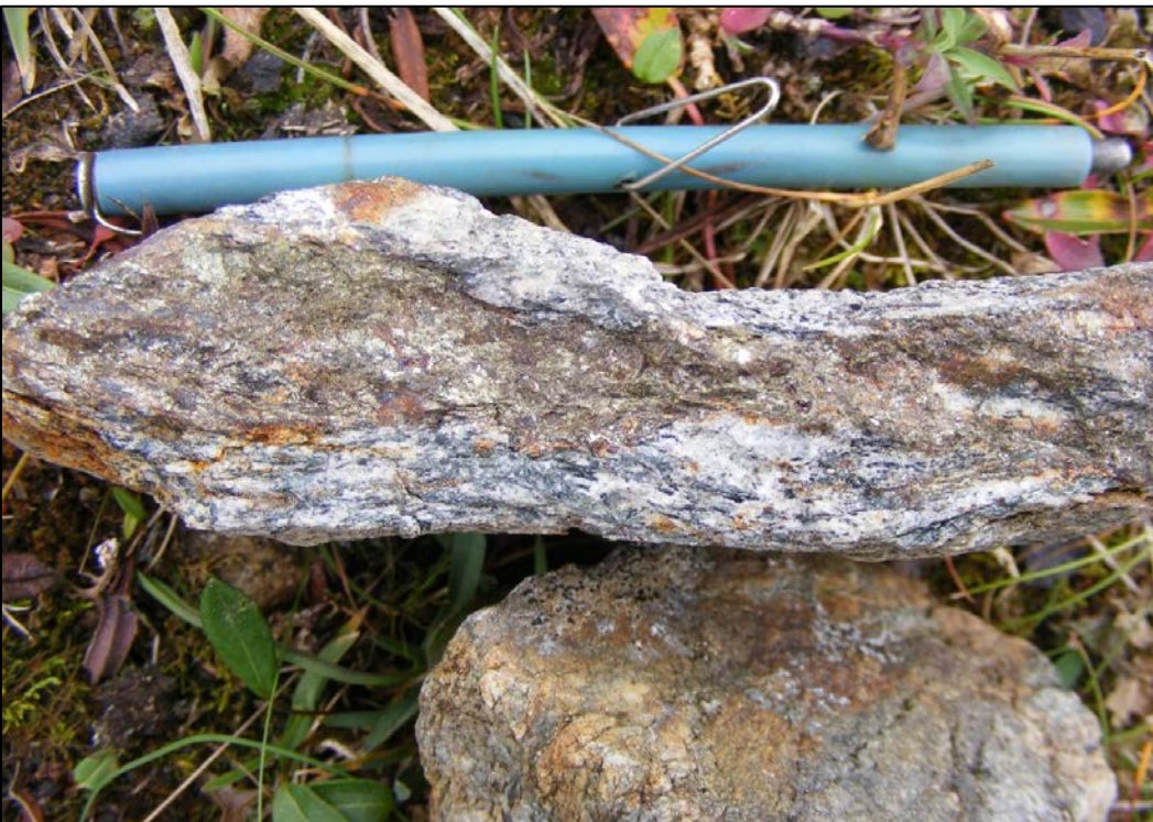
Figure 2: Foliated carbonate-amphibole rock with semimassive chalcopyrite band
