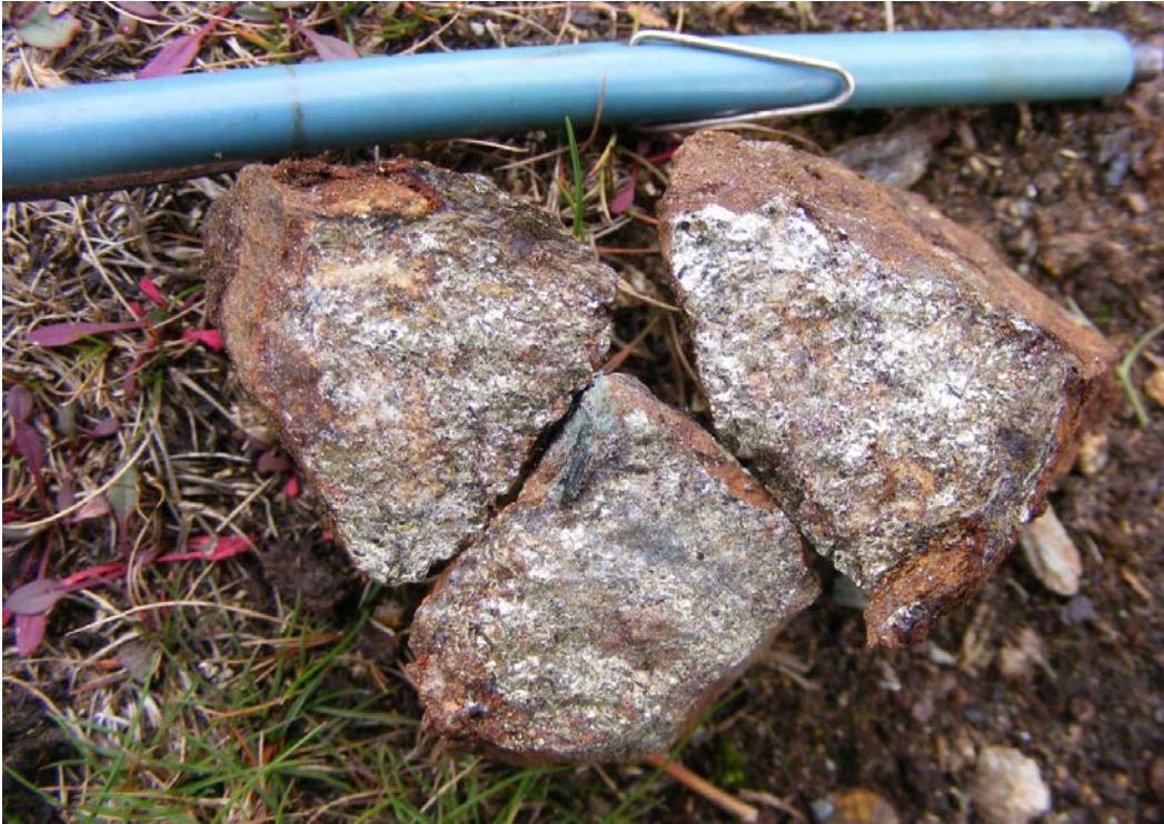
Figure 2: Foliated carbonate-amphibole rock with semimassive chalcopyrite band
